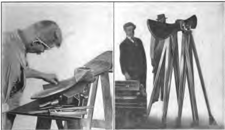
FIG. 21.—Testing shape of blade.
