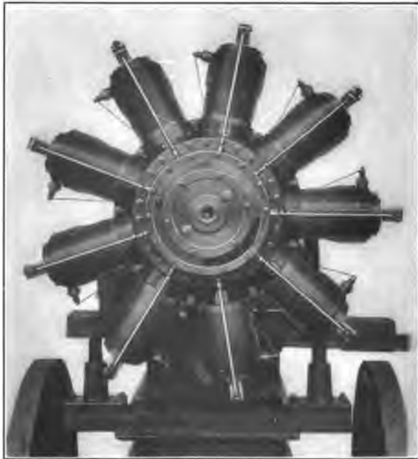
FIG. 86.—Gnome engine in test frame.
