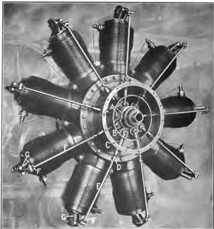
FIG. 88.—Cam action of Gnome engine.
