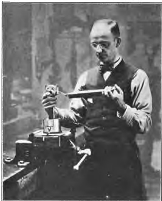
FIG. 63.—Fitting piston pin.
