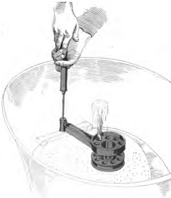
FIG. 98.—Cleaning and washing mother rod.
