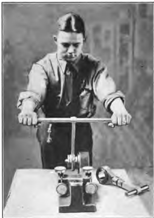
FIG. 64.—Straightening connecting rods.
